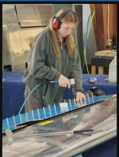
Reagan is riveting the final skin on the wing.
